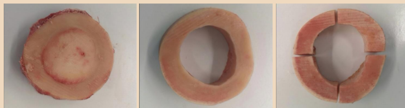
Figure 2 – The removed of soft tissue and trabecular bone from annulus before being sectioned into smaller specimens
